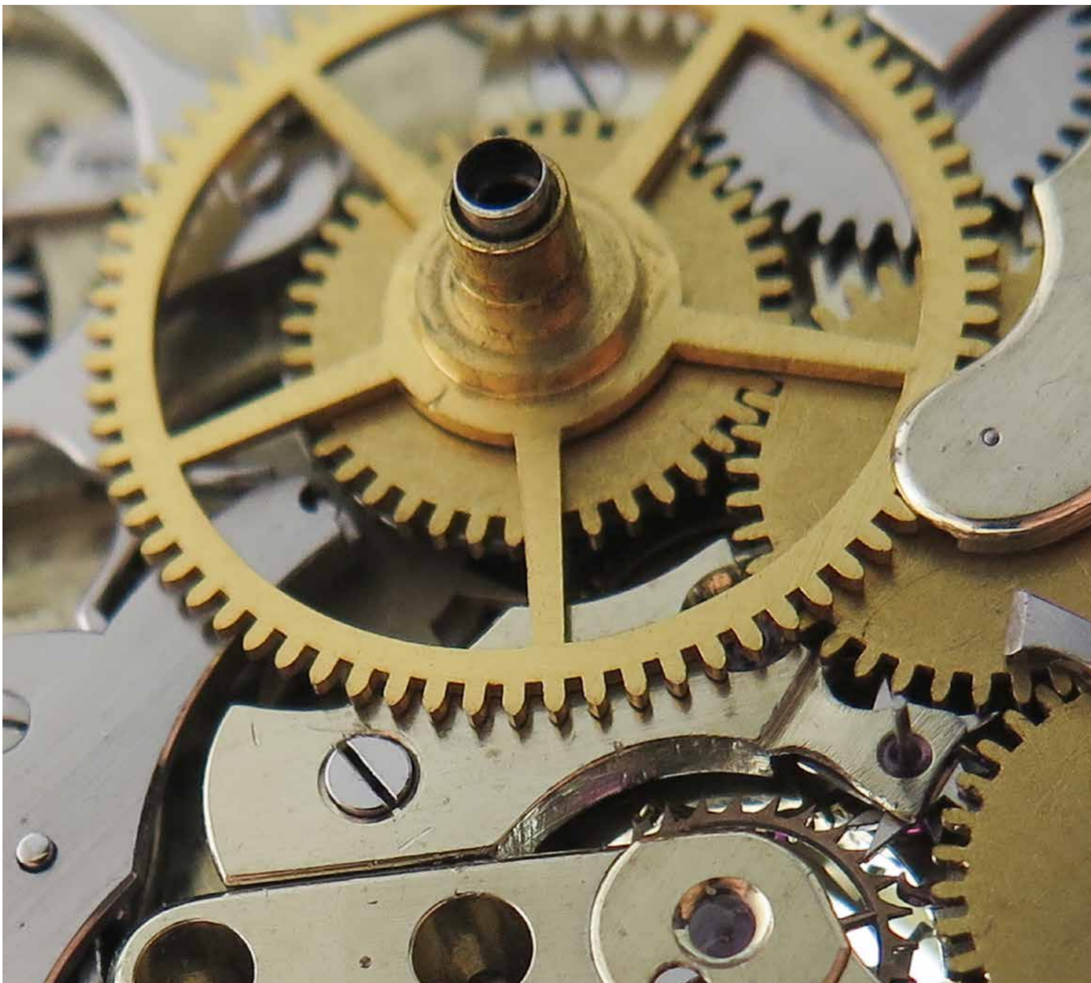
The oversized hour wheel. Larger in diameter than on the majority of movement constructions.
